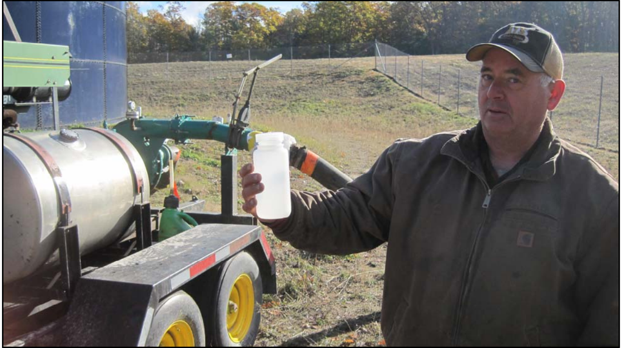
GRAB SAMPLE SENT TO A LAB FOR THE CADMIUM/PCB TESTING WHEN INJECTING FOOD ESTABLISHMENT WASTE (THIS RECENTLY WAS NO LONGER REQUIRED BY MDEQ)
