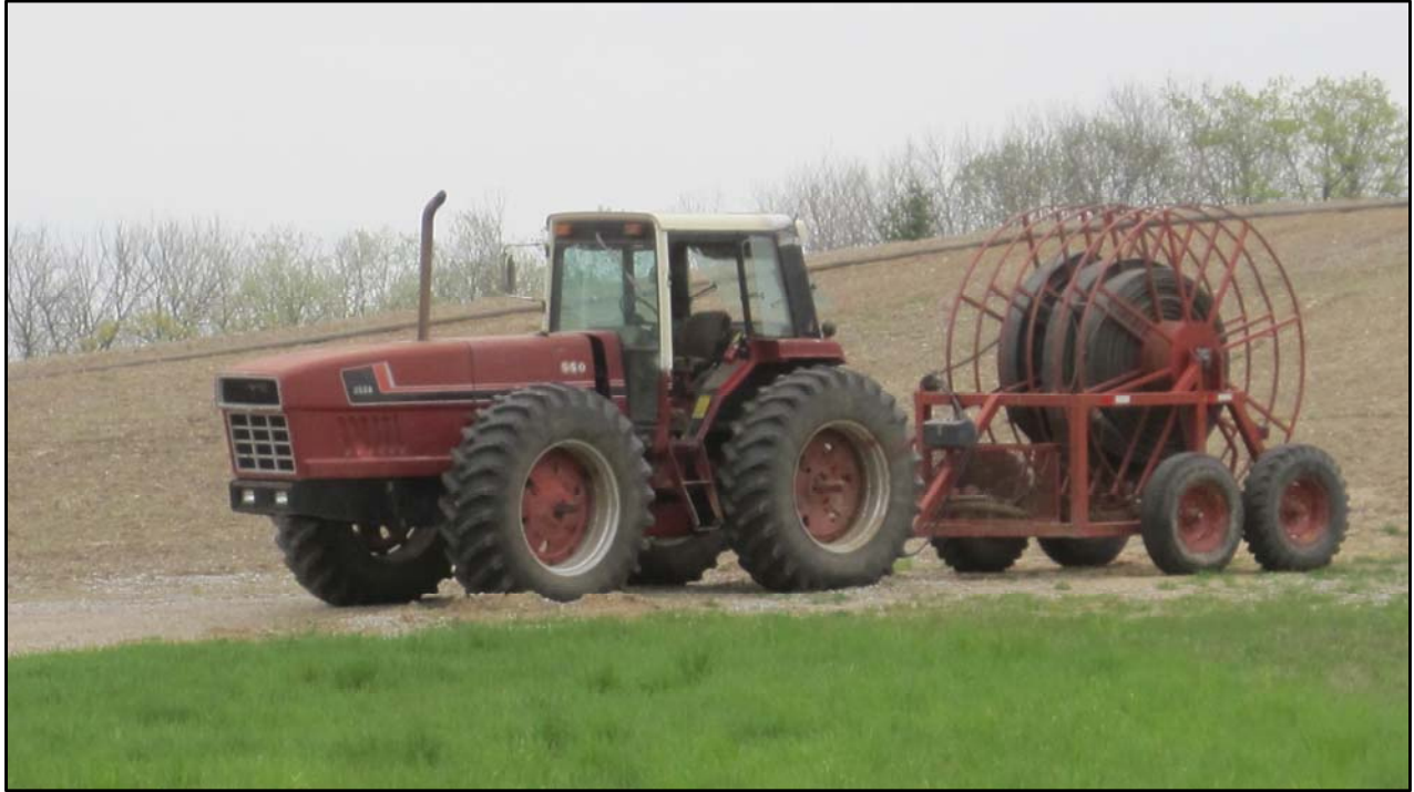
HOSE REEL USED FOR SETUP PRIOR AND AFTER TO INJECTION
