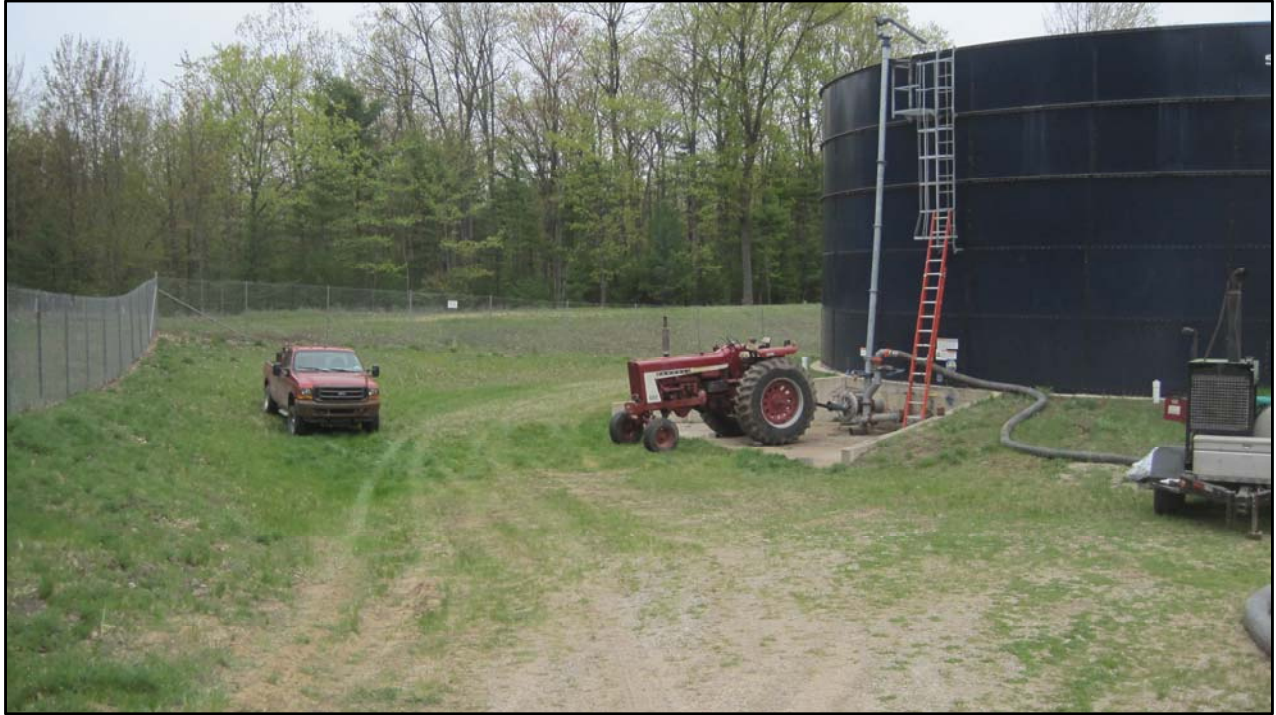
TRACTOR WITH PTO TO "SLURRY," OR HOMOGENIZE SEPTAGE WASTE PRIOR TO INJECTION
