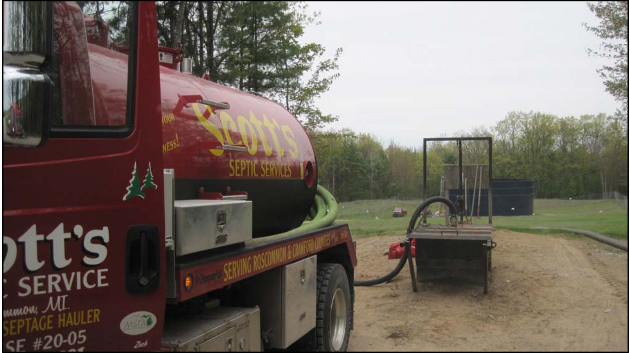
SLURRYSTORE IS FILLED FROM THE BOTTOM AS TRUCK IS OFF-LOADED THROUGH A BAR SCREEN
