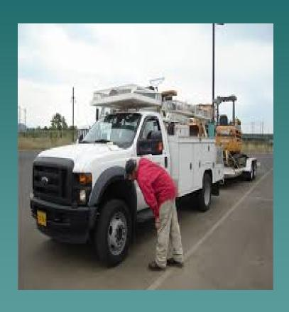
Check front of vehicle and check that low beams are on and both emergency flashers are working.
